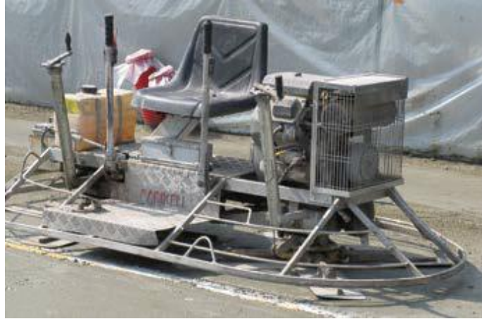
Figure 2-5: A double-rider (two rotors, each with blades) covering more area in less time than the walk-behind power machine.
