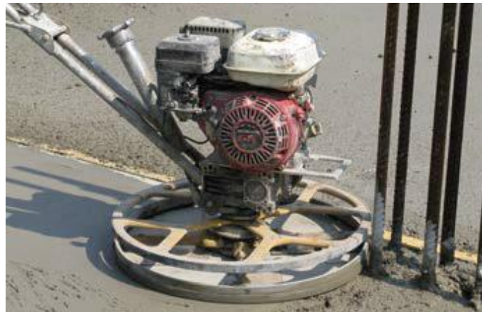
Figure 2-4: Power float equipped with disc for trowelling.
