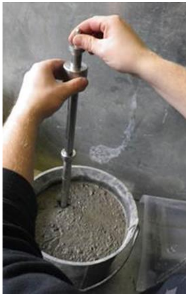
Figure 2-2: Determination of the beginning time for the finishing with the sonde Voton.
