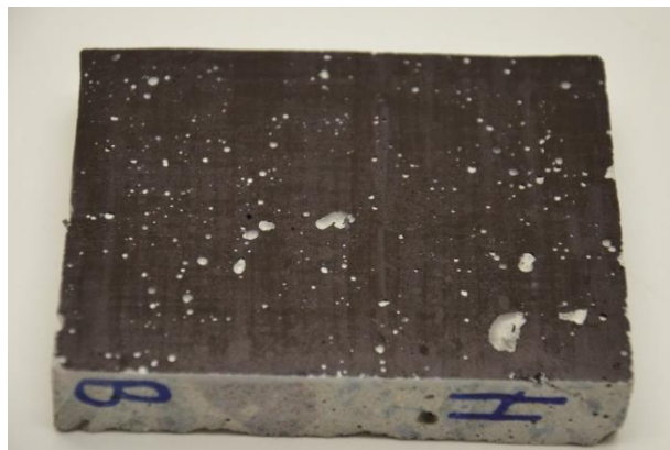
Figure 3-10: A prepared concrete sample for determining the air content.
