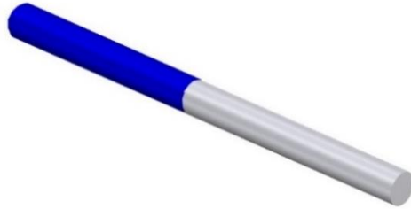
Figure 5-8: Dowel bar, half plasticized.
