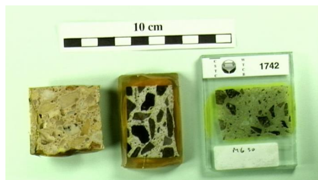
Figure 3-12: The different preparation steps for the making of a thin section.
