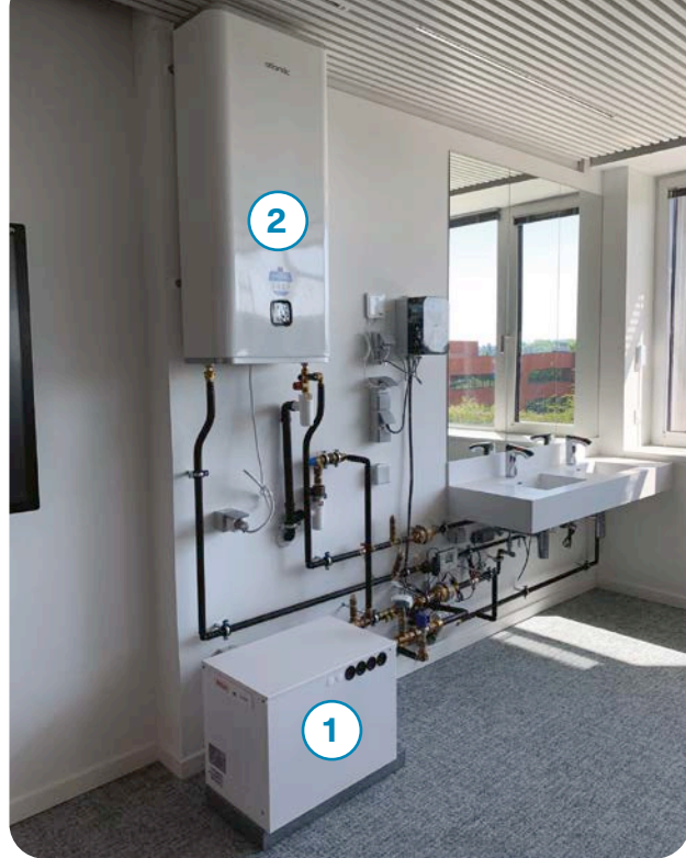
2 Test station where the performances of a PCM battery (1) are compared with those of an enamelled electric boiler (2).
