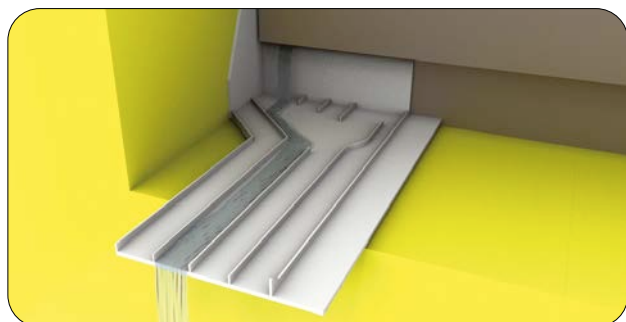
3 Drainage module consisting of preformed profiles with drip mouldings under the sill.
