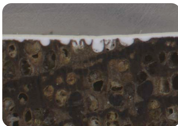
4 Application of two coats of primer: the pores are filled and the paint forms a continuous, regular and homogeneous coating.
