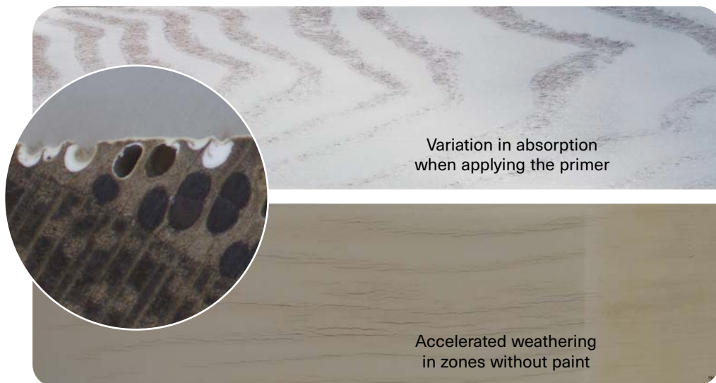
2 Example of over-painting coarse-pore wood without pore filler.
