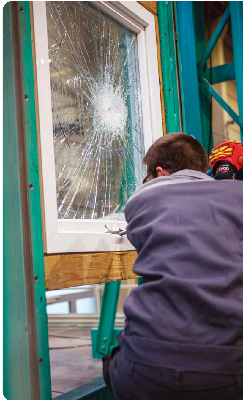
1 Intrusion test on joinery with resistance class RC 3 and glazing of class P5A.
