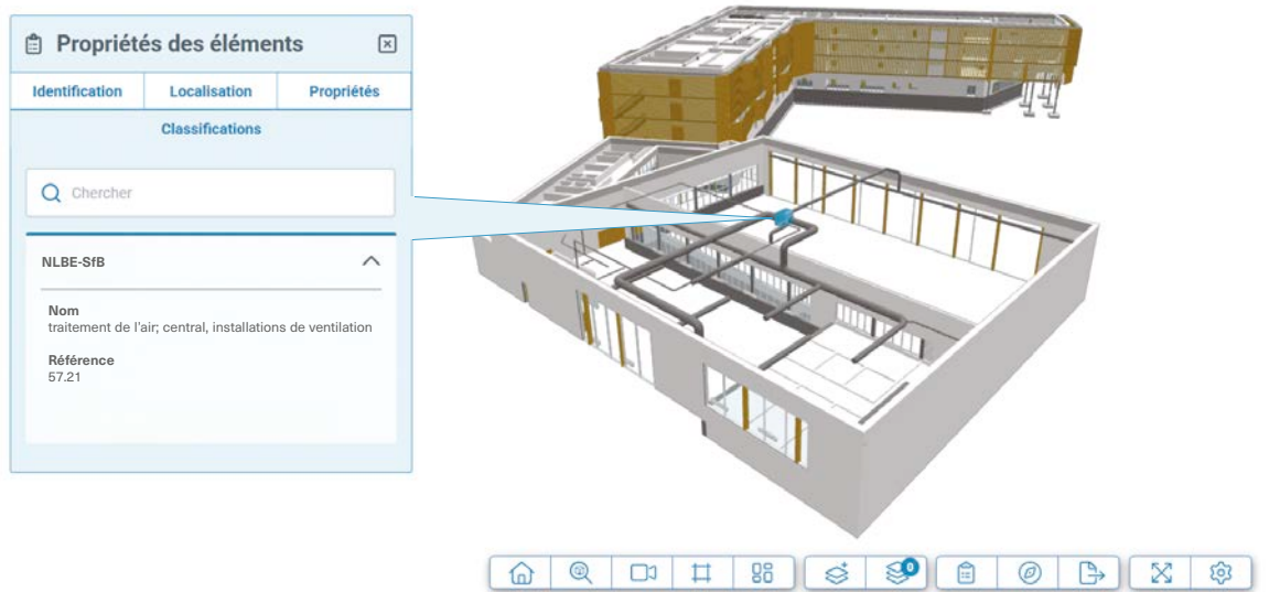
1 Air-conditioning plant with NLBE-SfB classification in a BIM model.
