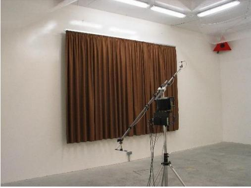
$$\alpha_s = \frac{0,16V}{S} \left( \frac{1}{T_2} - \frac{1}{T_1} \right) \quad [-]$$
