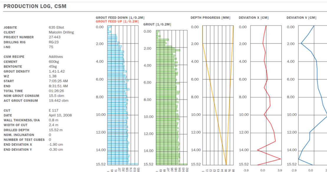
Figure 12: Typical production log (photo with courtesy of Malcolm Drilling Company)
