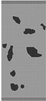
Figure 2. Mesh of the reference model (10% of surface area is composed of soil inclusions and the original observed shapes are used).
