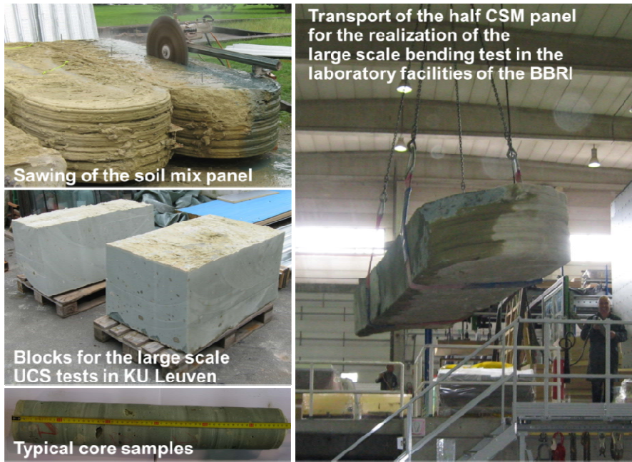
FIG. 5. Preparation of the test samples (cores, blocks and half panel) for the large scale mechanical characterization of the soil mix material
