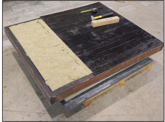
Figure 2. Construction of the dummy window
