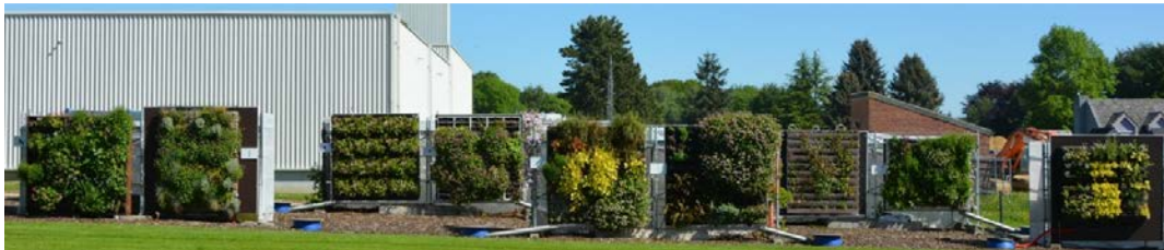
Figure 1 Picture of the test setup including nine Living Wall Systems
