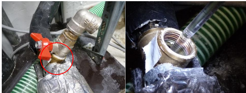
Figure 1: Picture showing how the dead water volume is collected using a sterile pipet
