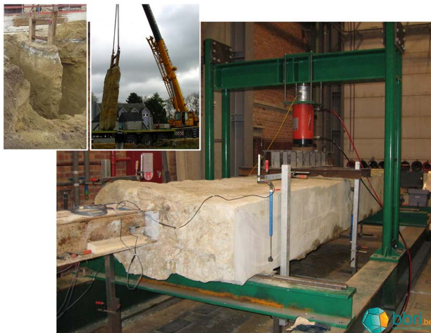
Figure 5. Large-scale bending tests performed on real-scale soil mix elements (columns or panels) within the framework of the BBRI Soil Mix project (2009-2013) [24, 25].
