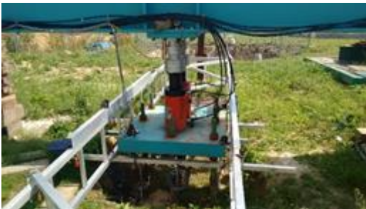
Figure 4. Micropile group instrumentation
