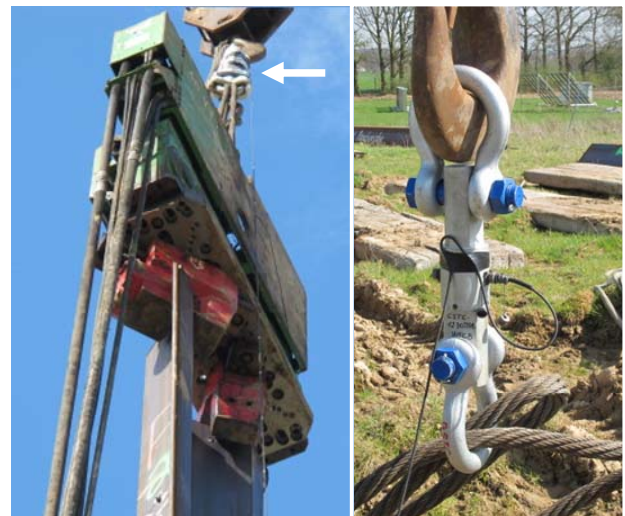
Figure 4. BBRI holding back force transducer as used during the test campaign
