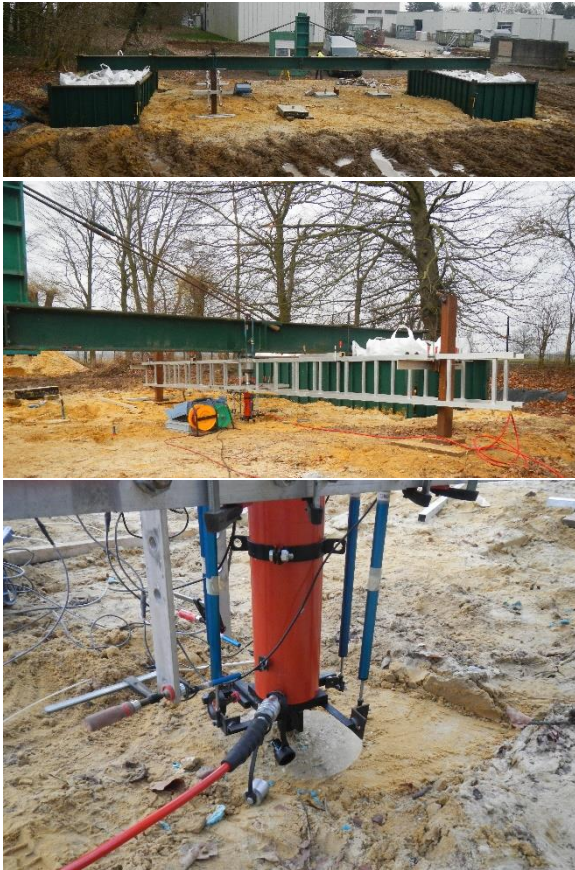
Figure 9. Different views of the reaction device and the measurement set-up used for the SLT's
