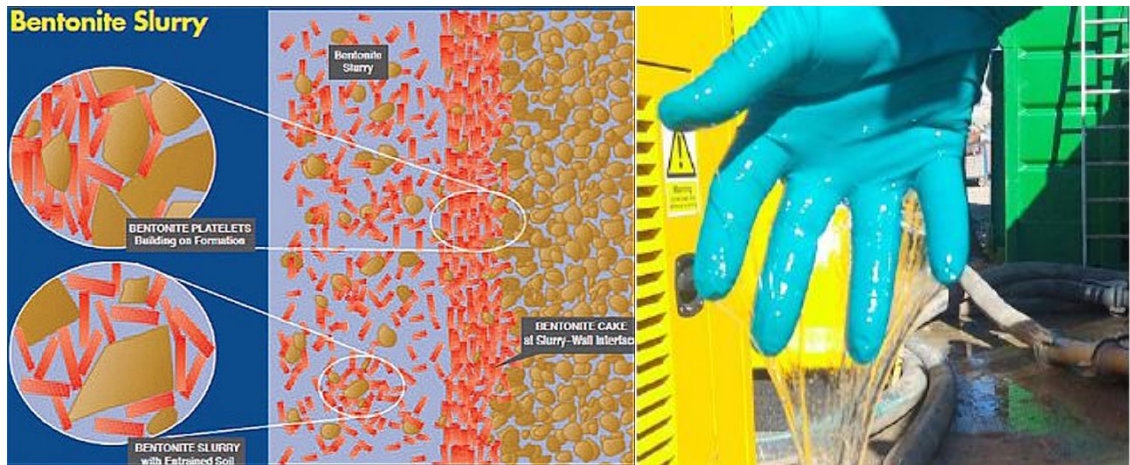
Figure 31. Comparative behaviours of bentonite and polymers
