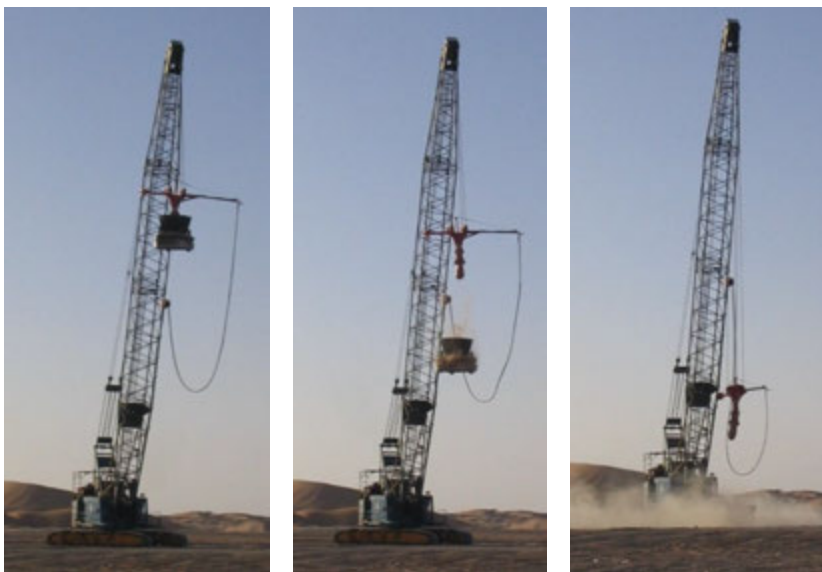
Figure 3: MARS automated drop and grab system
