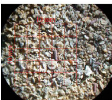
Photo 1: Sand sample (size of the grid is 10 mm)
