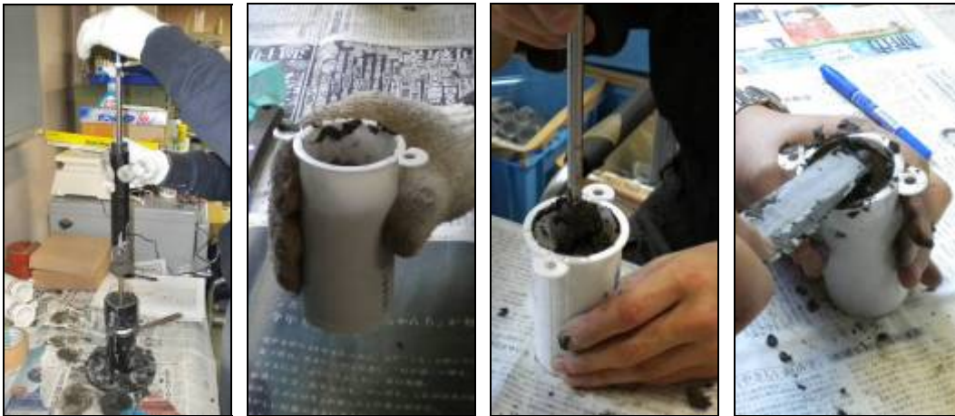
Photo 1: Molding techniques used, from left to right: Dynamic Compaction, Tapping, Rodding, No Compaction.
