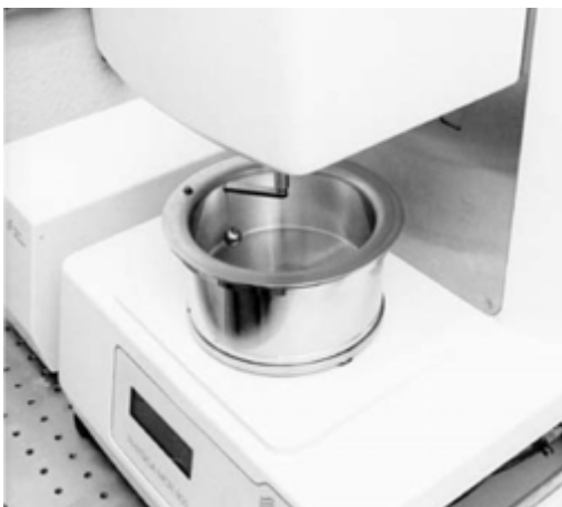
Figure 3: The BMS of Müller et al (1999) implemented in a standard rheometer (Schatzmann et al, 2009).
