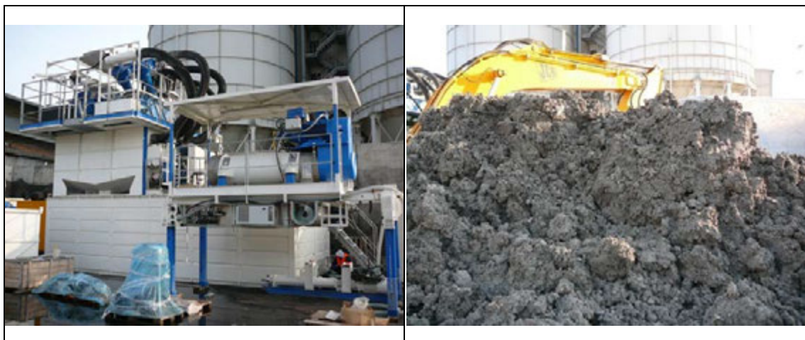
Photo 4: Treatment plant – Thickened silty and clayey fraction coming out from the centrifuge
