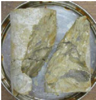
a, 8_TRI(25)_N Slickensides on failure surface
