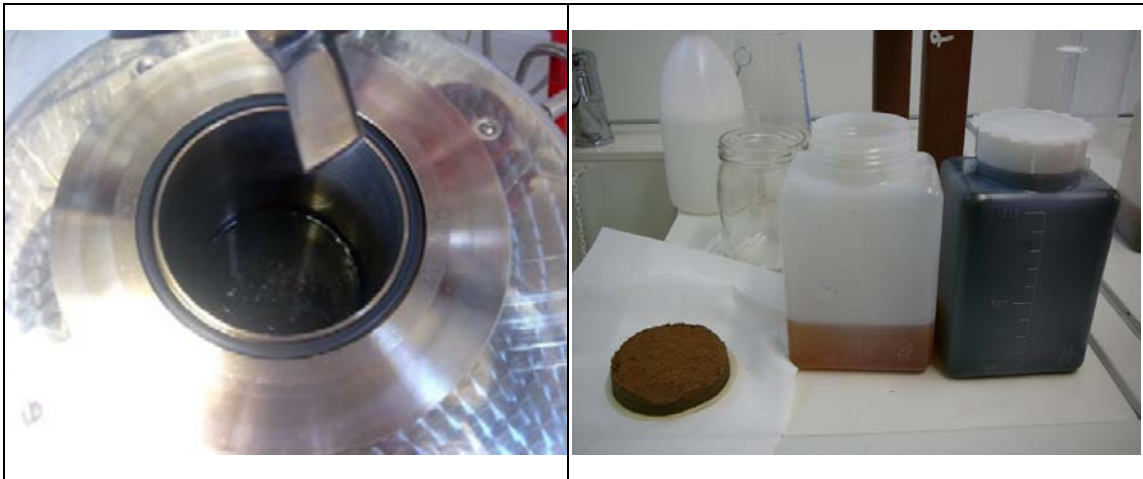
Photo 5: Loading of the pilot system Wet Oxi – Fractions entering and coming out of the Wet Oxi
