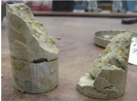
c, 32_TRI(75)_N. Wavy failure plane
