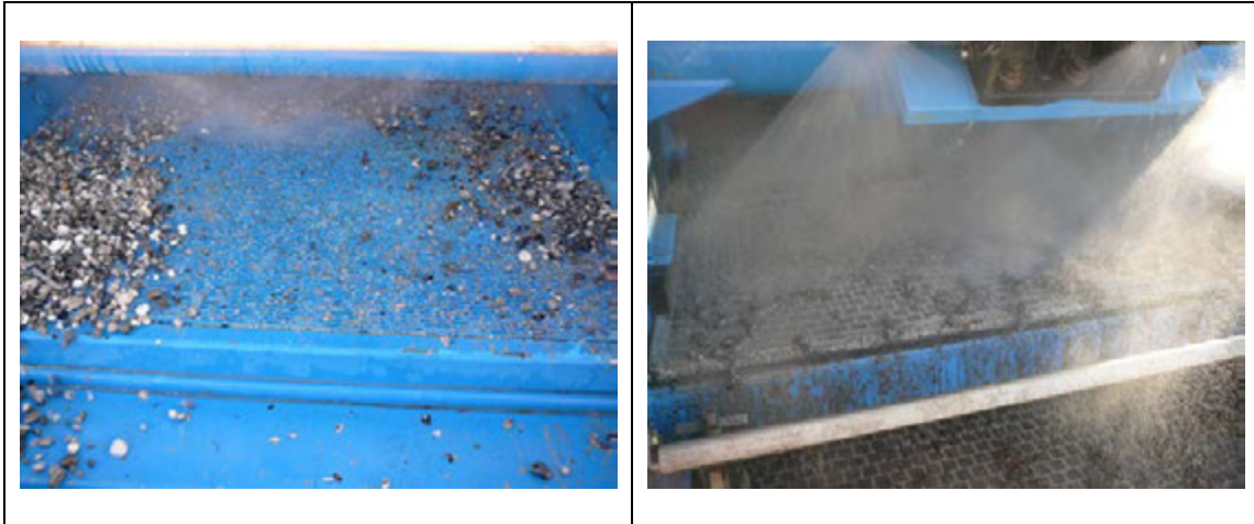
Photo 2: Coarse solids being washed on the refining sieve and sandy material being washed in the secondary sieve.
