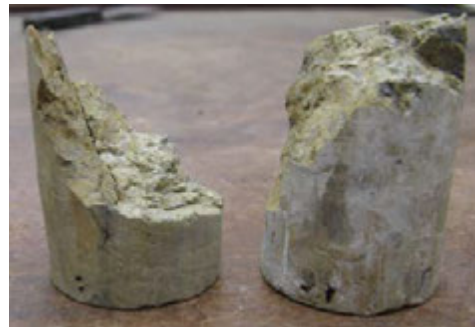
d, 32_TRI(50)_L Curving failure plane
