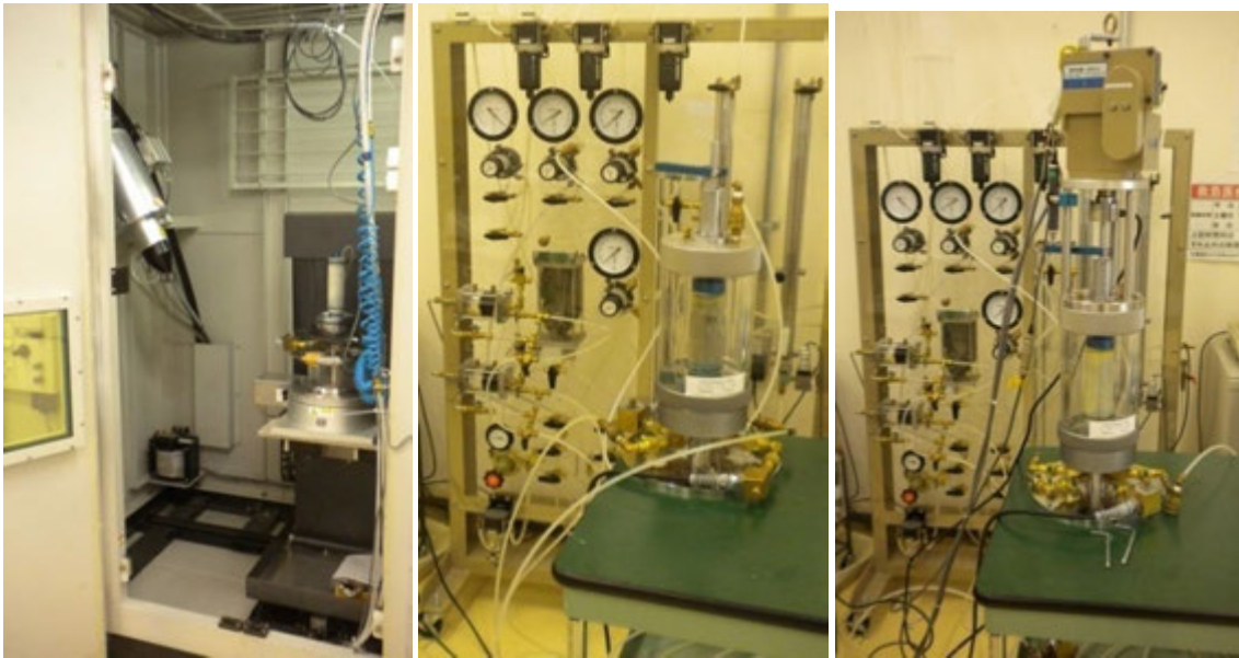
Photo 2: From left to right: X-Ray CT scanner, Triaxial apparatus and press used.
