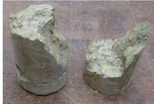
b, 32_TRI(25)_L Abrupt change in failure plane
