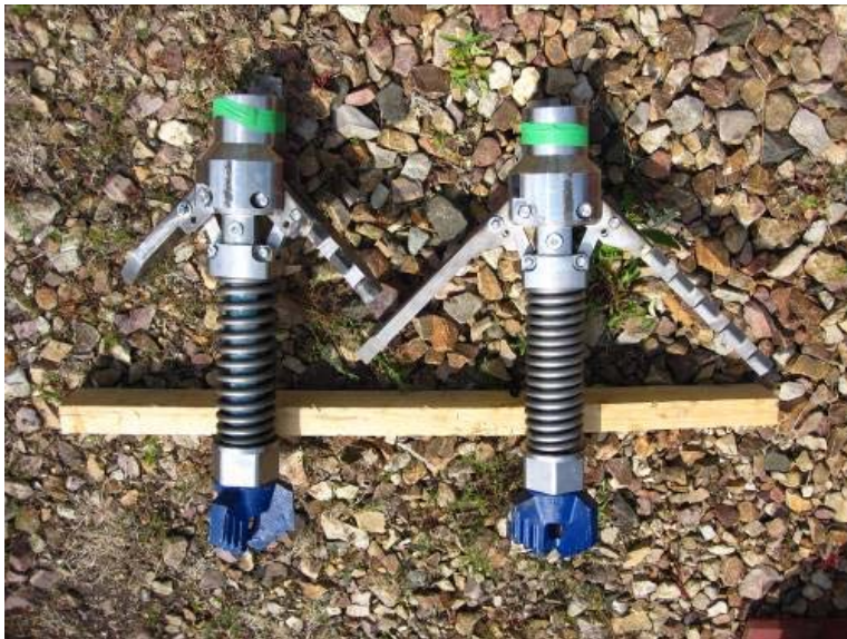
Photo 1: Springsol mixing tools (400 mm (left) and 600 mm (right) diameters).
