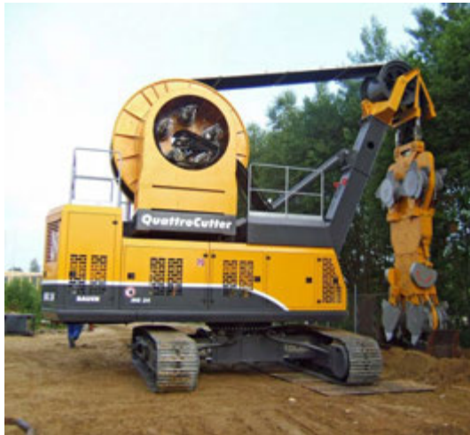
Photo 3: Wire rope-suspended CSM unit, QuattroCutter, Germany
