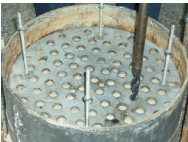
Photo 2: Clay is drilled with aid of prebored steel plate and auger
