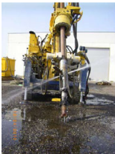
Figure 2: New soil-mixing folding tool FLAPWINGS
