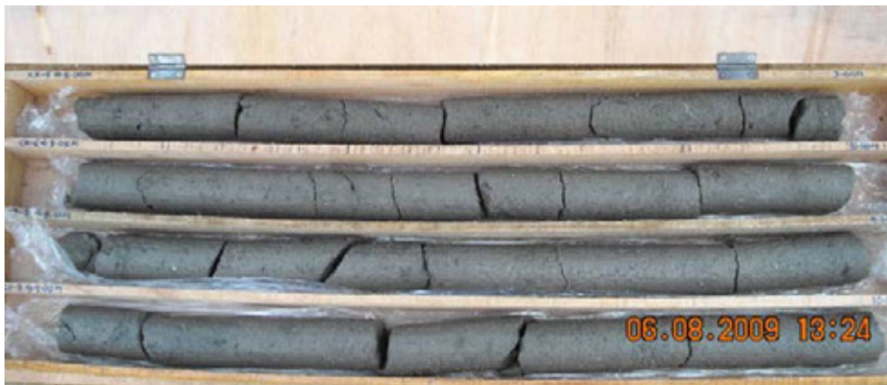
Figure 10: Cored Sample of a well-constructed and uniformly treated DSM column
