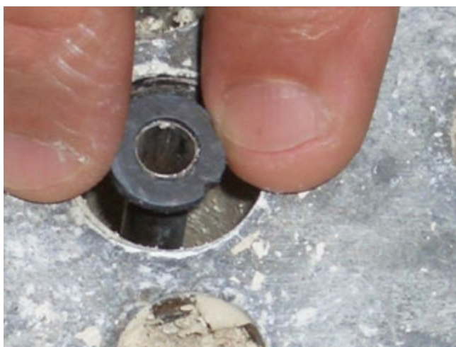
Photo 1: Placement of ring type magnet to the antenna rod
