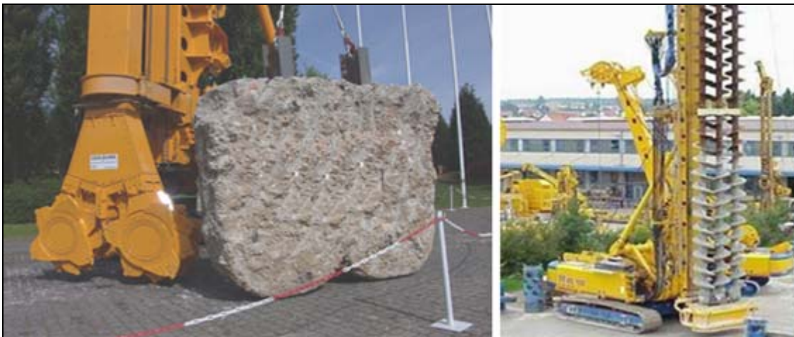
Figure 9: View of the CSM equipment and a CSM panel (on the left) and the equipment used in DSM technology (on the right).
