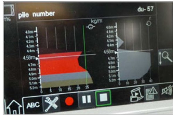
Photo 11: PDE screen, visualisation of the column production
