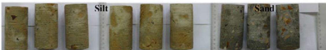
Photo 4: Specimens cored from block samples of columns X4 – X5 and X6.
