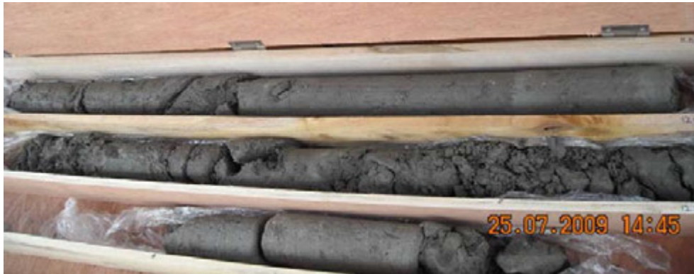
Figure 11: Cored Sample of a poorly constructed and non-uniform DSM column
