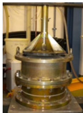
Figure 4: Consolidation of the slurry in a container
