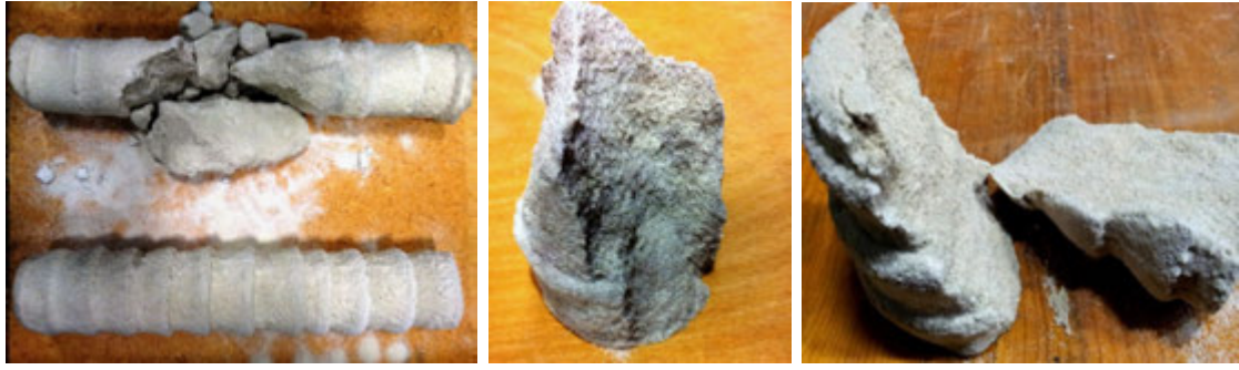
Figures 6a-6b-6c: on the left, unloaded column and damaged column from test 2 - in the middle, failure of SM specimen taken from test 2 after a UCS test- On the right, failure of SM specimen taken from test 3 after a UCS test.
