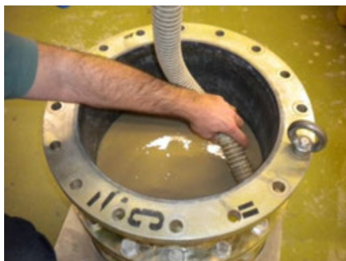
Figure 3: Pouring slurry into the container
