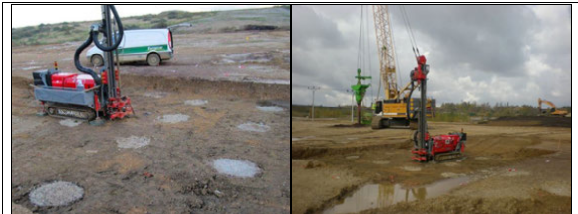
Photo 6 : Execution of the Ménard pressuremeter
