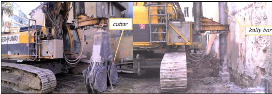
Figure 9: Components of the equipment: cutter head and kelly bar.
