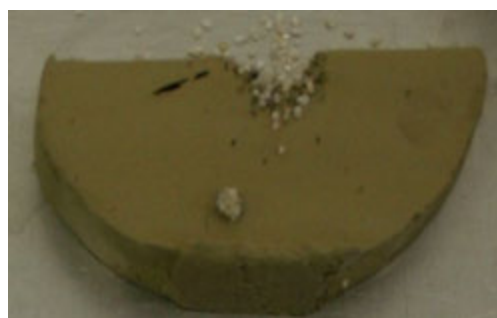
Figure 9: Typical MIP sample
