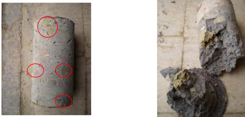
Figure 13: Photos of soil-cement samples before and after UCS tests
