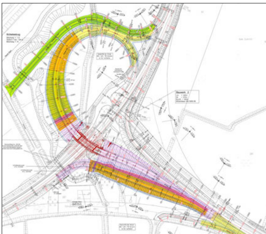
Figure 1: project overview: crossing highways B5 and B202 (CMC close to bridge and coloured areas with vertical drains and preloading)
