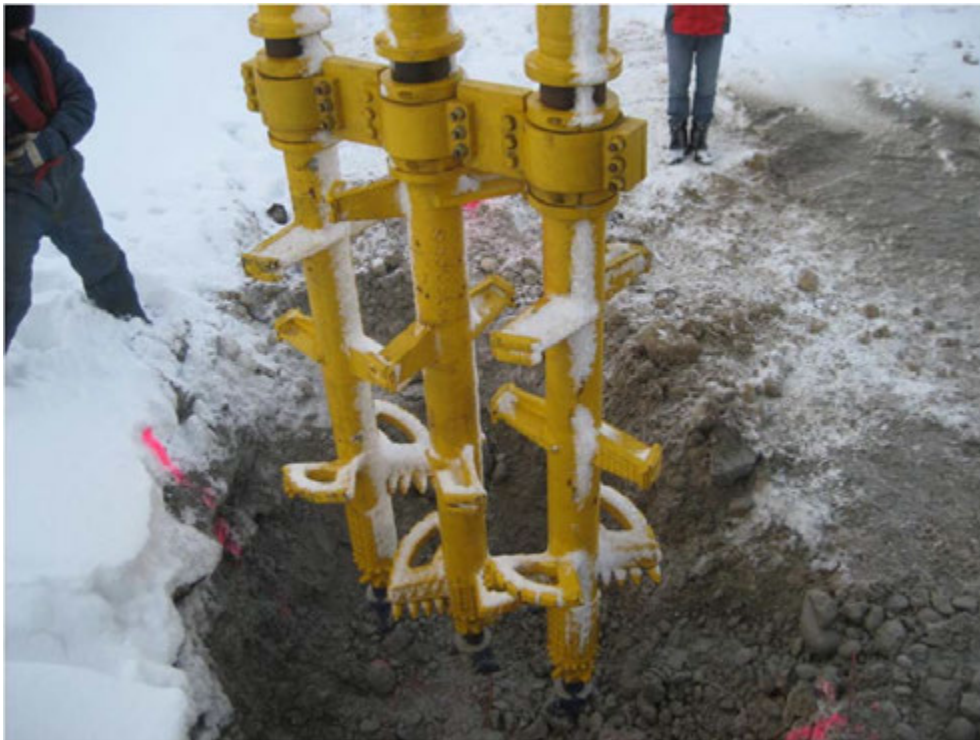
Photo 1: DSM Mixing tool with three mixing shafts (property of Keller Grundbau GmbH)
