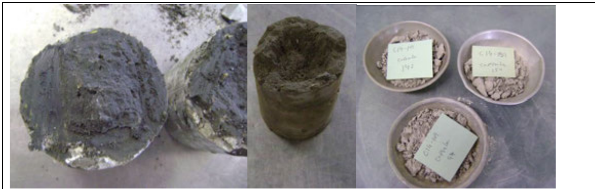
Photo 4: Water content determination of cylindrical specimen preparation after unconfined compression test
