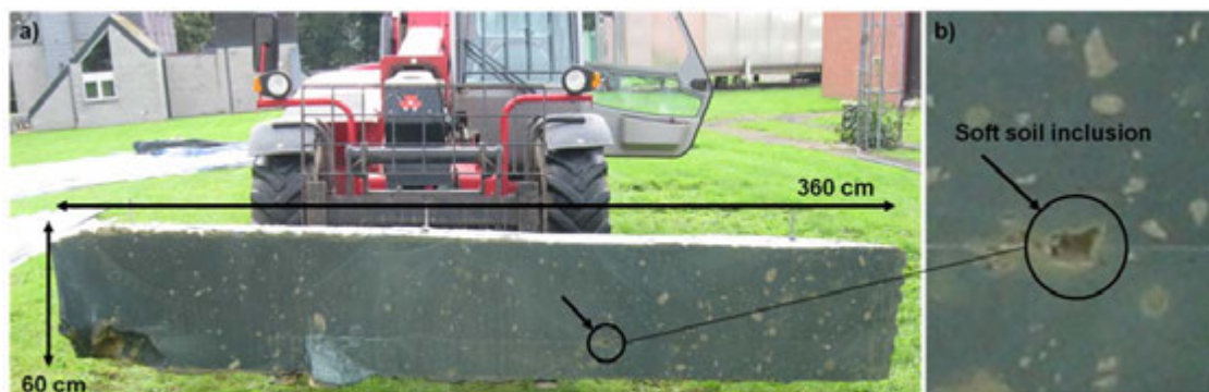
Figure 2: a) Saw-cut section of a CSM panel, b) enlargement of a soft soil inclusion
