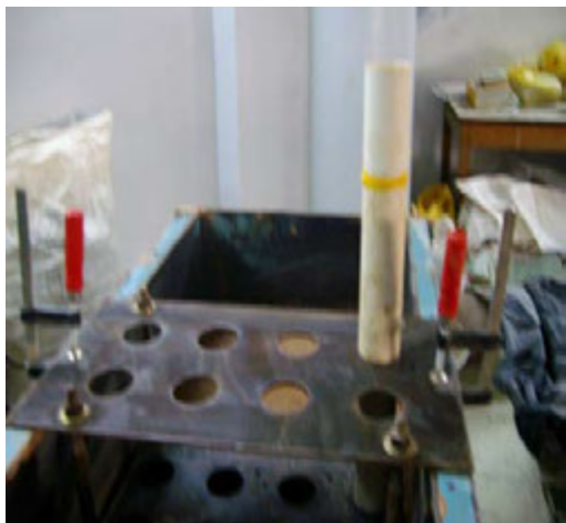
Photo 1: Construction of encased stone columns
