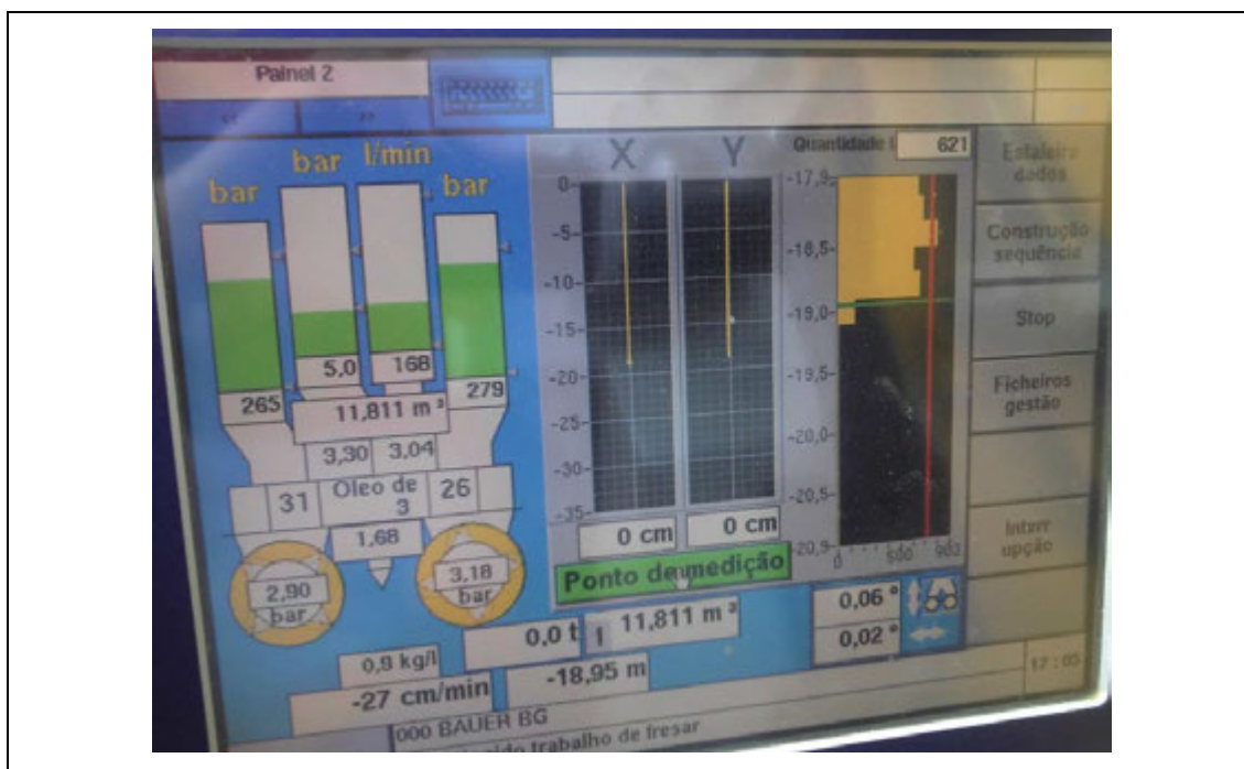
Figure 12: Rig operator’s monitor to control of the execution parameters.
