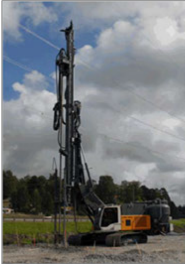
Photo 4 and 5: LRB 125 XL during column production
