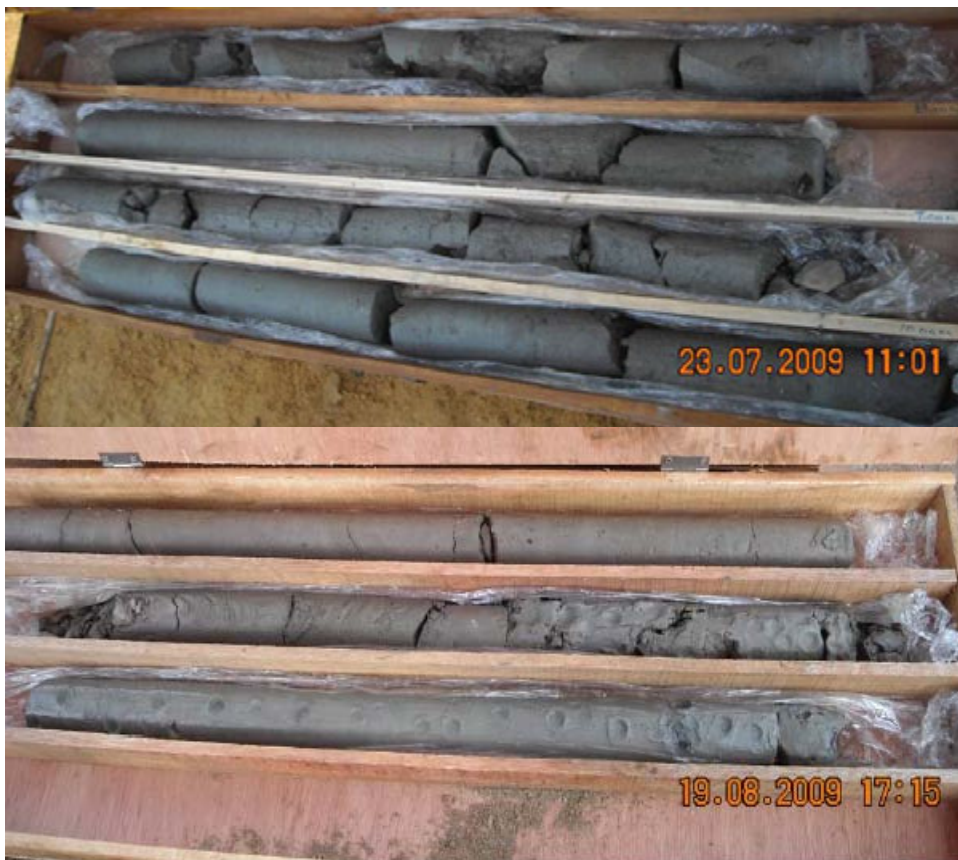
Figure 8: Coring Samples Photo showing some inconsistent results
