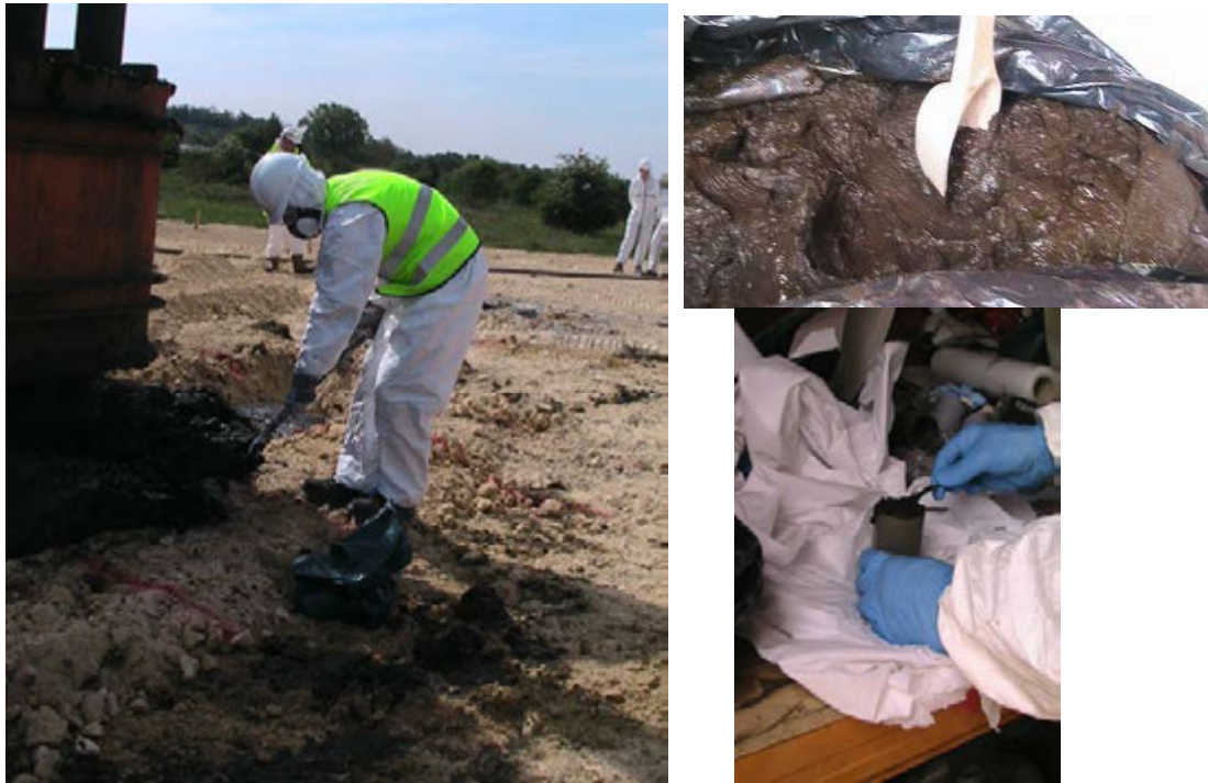
Figure 10: Surface sampling of the various installations during construction and sample preparation.
