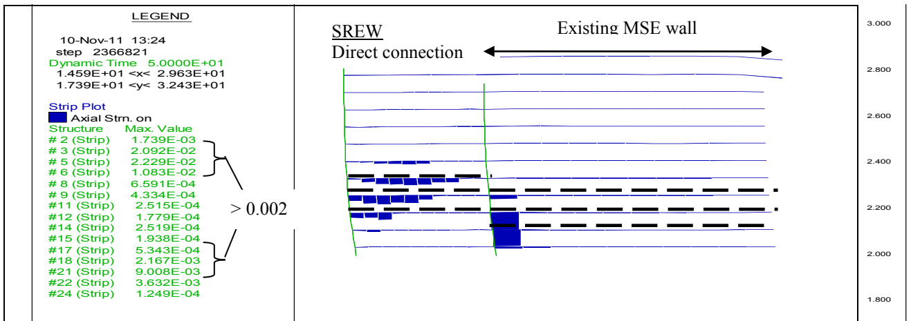
Figure 11b: Strain in soil reinforcement in existing MSE wall SREW with Direct Connection. The strips with strain beyond the elastic limit are shown in bold dotted line
