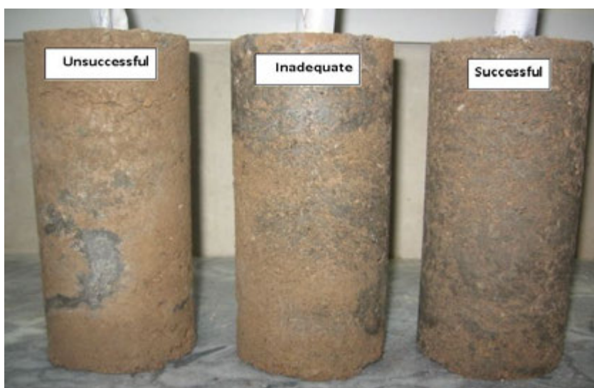
Figure 4: The schematics of grouting results of the three samples: successful, inadequate, and unsuccessful
