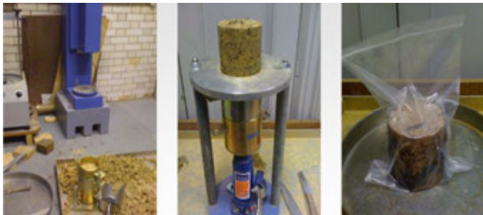
Photo 2: Reinforced sample compaction procedure
