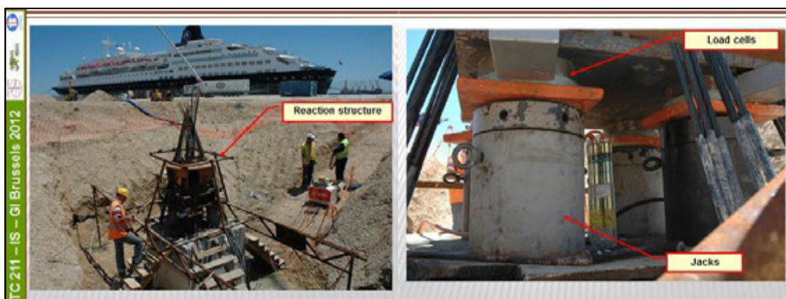
Figure 12: Vertical full scale load test: reaction structure and load applying system.
