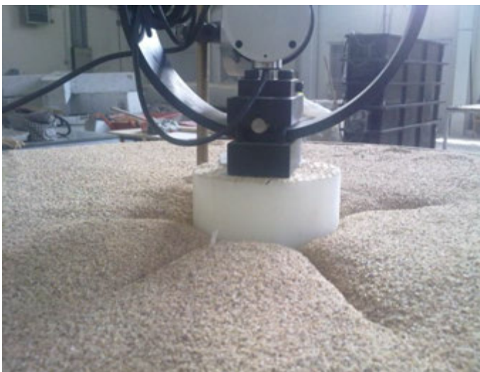
Photo 2: Shear Failure Pattern Appeared at the Surface for Relative Displacement S_v/D of 20%
