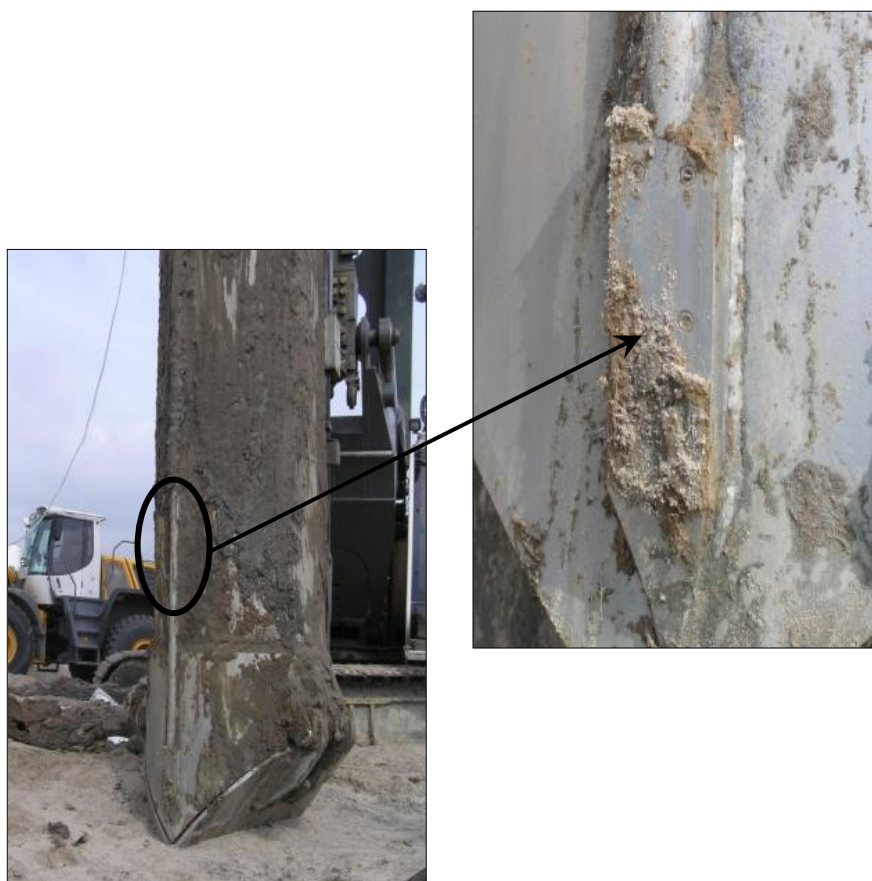
Figure 16: Displacement pipe equipped with measurement instrumentation to record acoustic signals
