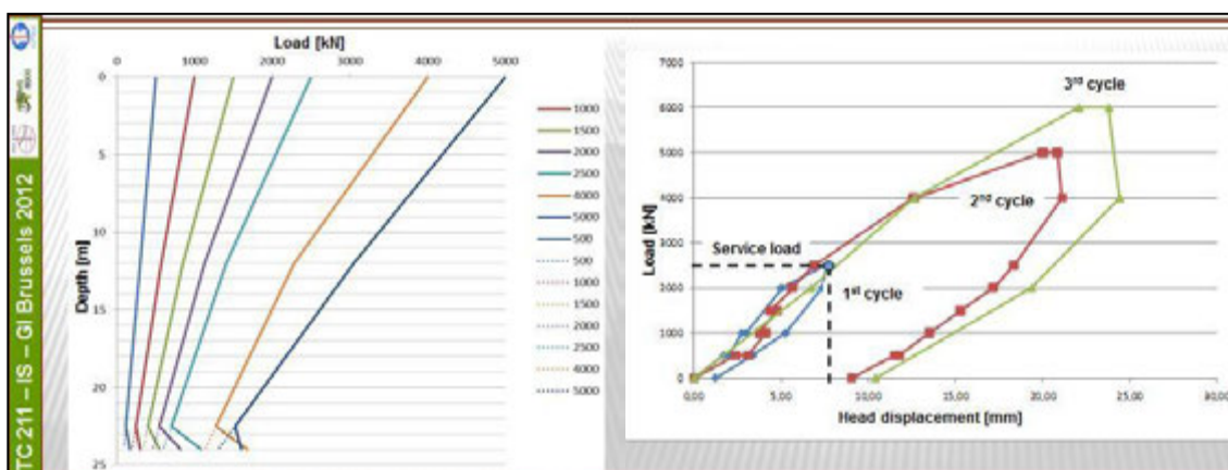
Figure 13: Vertical full scale load test: main results.
