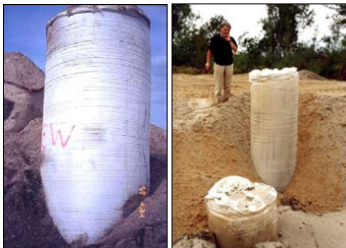
Figure 3: Demonstration of the confining capability of high strength geotextile encasement for GEC “in air”
