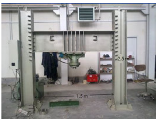
Photo 1: Loading Apparatus Implemented in the Study
