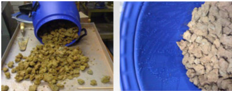
Photo 1: Chopped clay peds in storage drum
