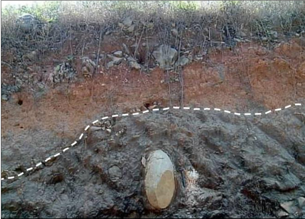
Figure 12: Soil profile with completely weathered rock (laterite, above dotted line) on top of (partly) weathered rock (below dotted line)
