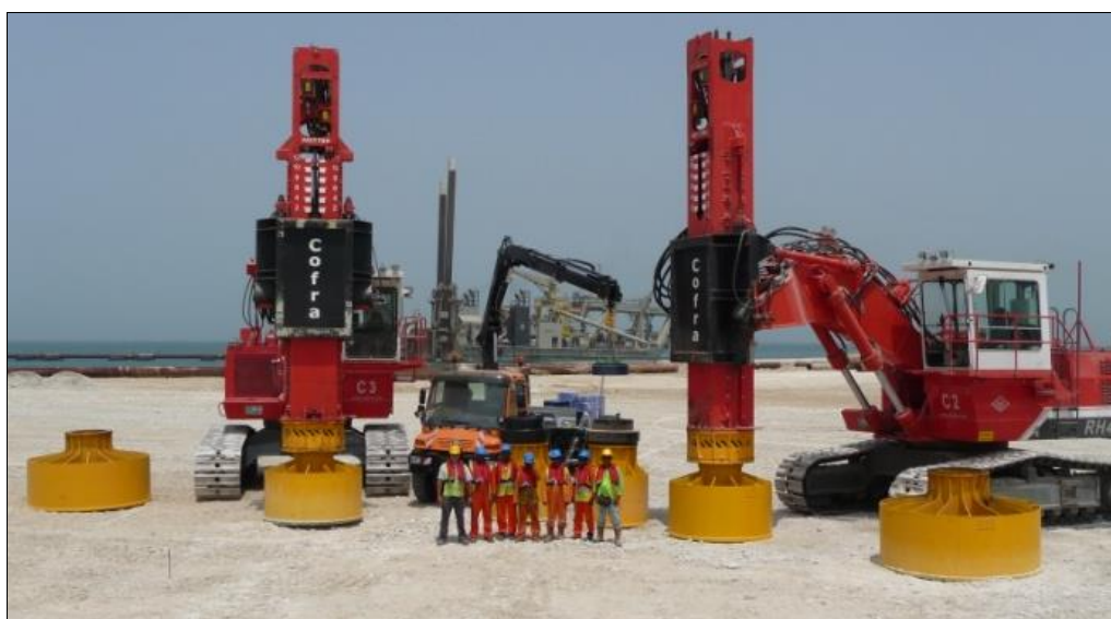
Figure 19: Rapid Impact Compaction equipment (Cofra Group)
