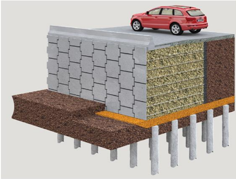
Figure 40: Combination of MSE-wall with soil reinforcement
