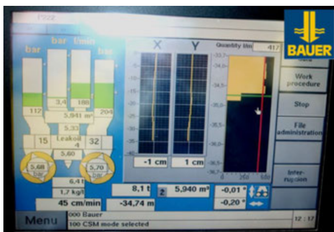
Figure 59: Equipment overview of the CSM – real time representation of the monitored data, from Gerressen (2012) with the courtesy of Bauer
