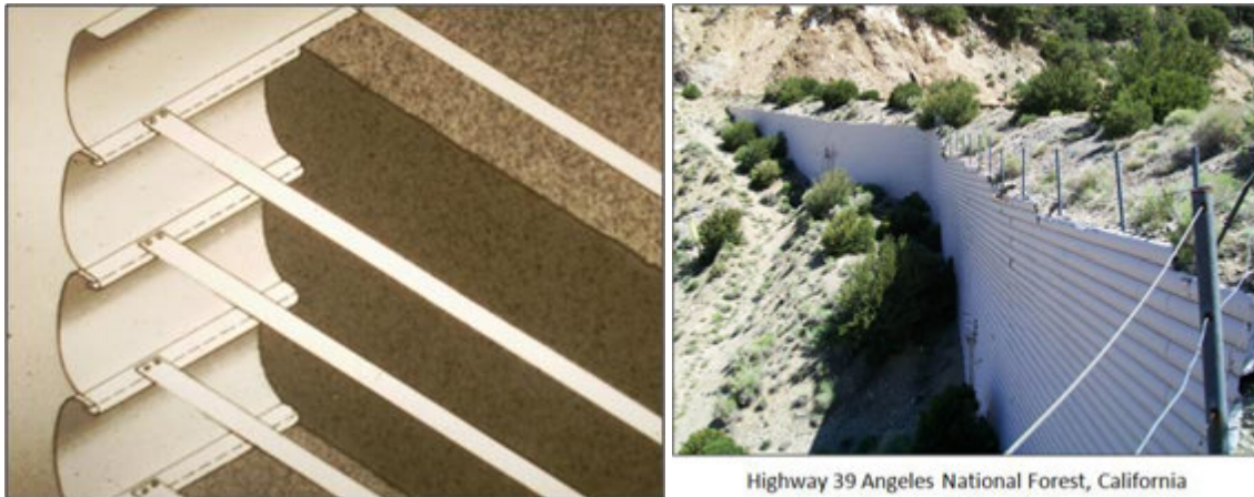
Figure 28: Concept of original Terre Armée
