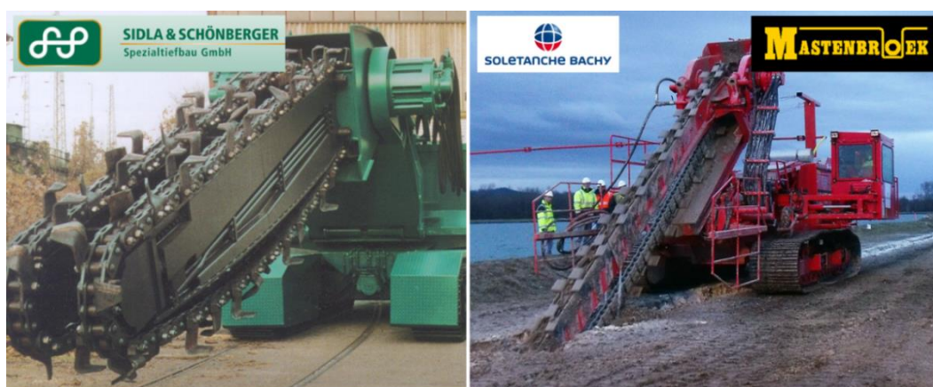
Figure 15: Trenchmixing tools, from Topolnicki (2012) with the courtersy of Siedla-Schönberger and Soletanche-Bachy/Mastenbroek
