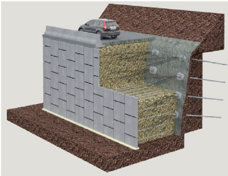
Figure 41: Combination of MSE-wall with soil nailing
