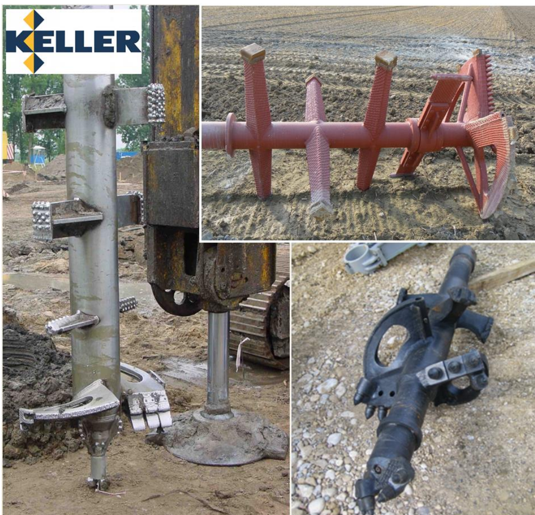
Figure 5: Keller wet soil mix system in single shaft configuration (available tool diameter for single shaft ranging between 40 and 240 cm), after Topolnicki (2012) , with the courtesy of Keller
