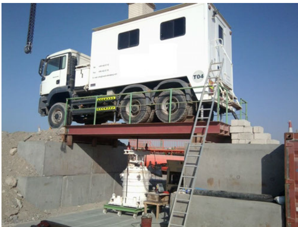
Figure 61: Typical set-up for onsite calibration chamber testing
