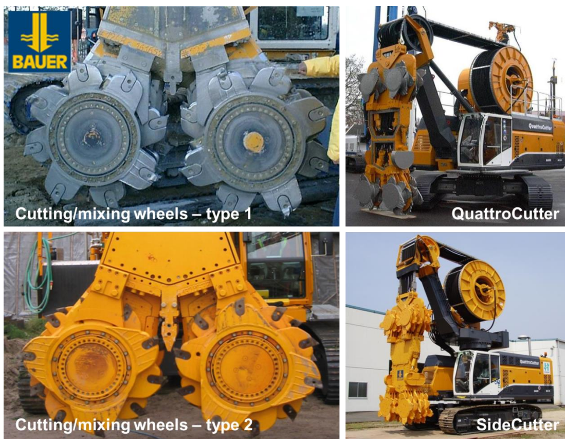
Figure 13: The cutting/mixing tools of the Bauer CSM system (on left) and the QuattroCutter and SideCutter systems, from Gerressen (2012) with the courtesy of Bauer
