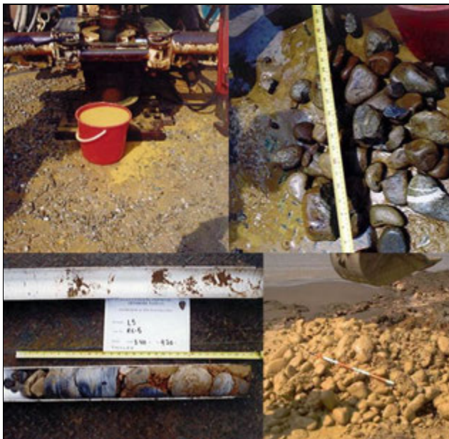
Figure 10: Sampling results in mixed soil unit by applying different techniques; air flush percussion drilling (left, top), air-water flushing at high flow rates in larger casings (right, top), diamond impregnated split double tube core barrel (left, bottom), sample with backhoe (right, bottom)
