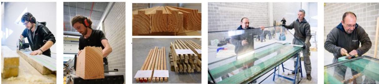
Figure 2. Wood and glass preparation before reuse
