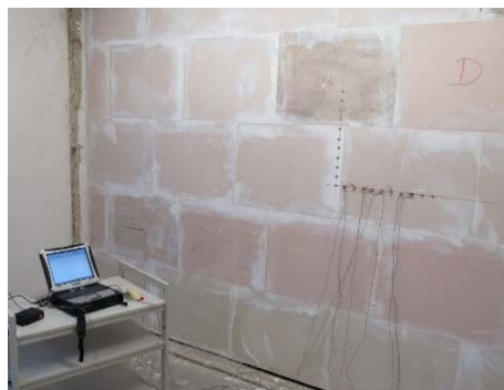
Figure 6 – Picture of the gypsum block wall and the horizontal line of accelerometers
