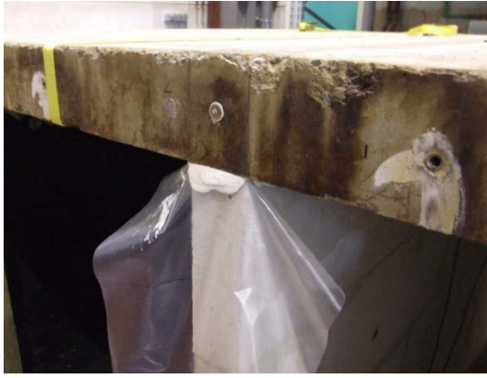
Figure 9: Picture of the use of the plastic sheet - The vertical walls are composed of cellular concrete ( \rho' = 46 \text{ kg/m}^2 )
