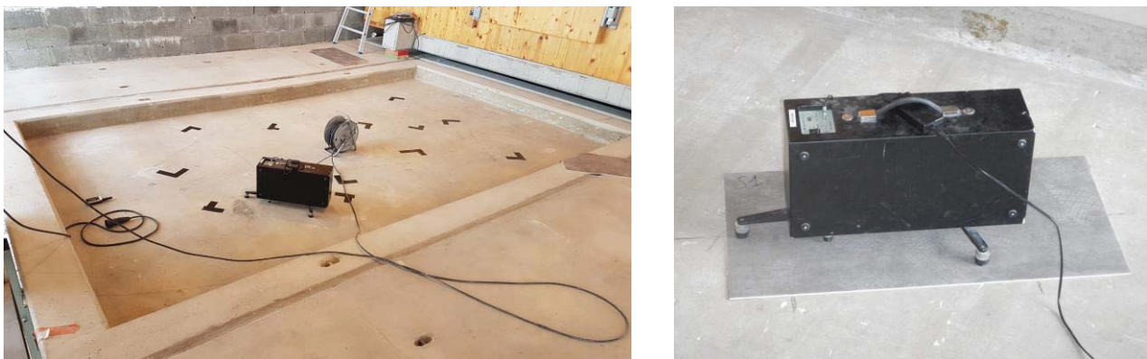
Figure 2 – Impact sound insulation measurement of bare floor and bare floor with vinyl floor covering
