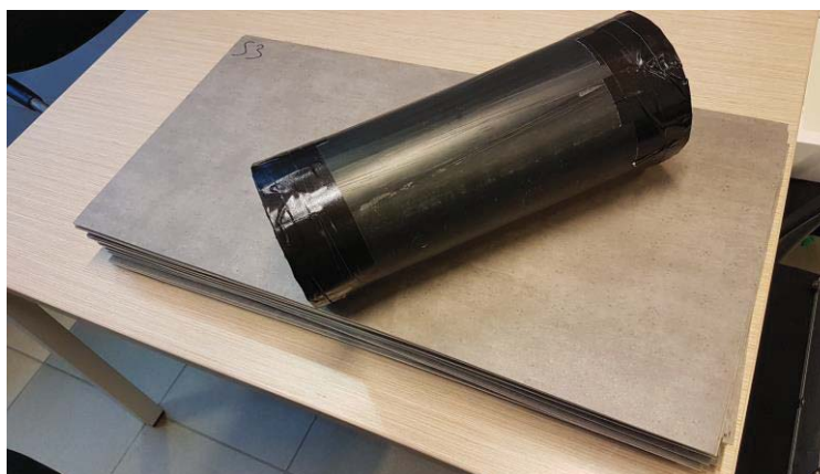
Figure 1 – Vinyl floor covering test samples sent to the participating laboratories.
