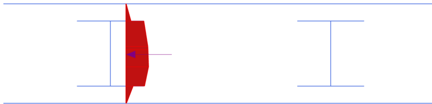
Fig. 6. Shear stress distribution, \tau_s , developing along the cross-section at the boundaries of the flanges of the steel beam (for f_{sm,tk} = 0.1 MPa)
