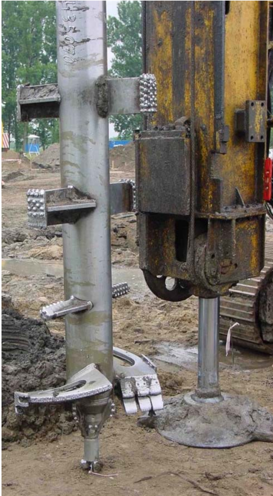
Fig. 7. Picture of a drilling/mixing head used for the execution of soil-cement columns in single shaft configuration (with the courtesy of Michał Topolnicki - Keller)
