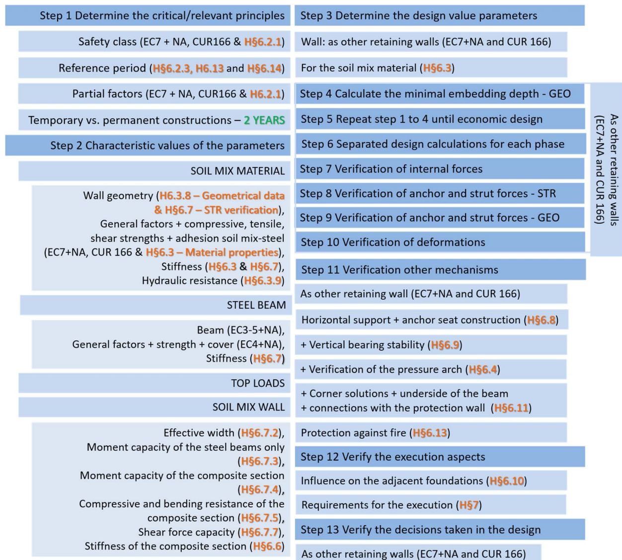
Fig. 26. Flow chart for the design of a soil mix wall used as retaining wall (according to the handbook) – “H”, in the figure, means BBRI/SBRCURnet Handbook Soil mix walls (2018)
