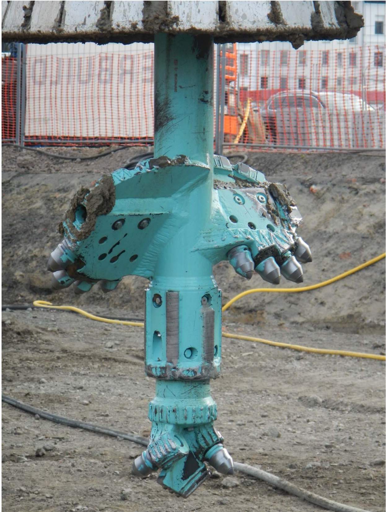
Fig. 8. Picture of a drilling/mixing head used for the execution of soil-cement columns in single shaft configuration (with the courtesy of ABI)
