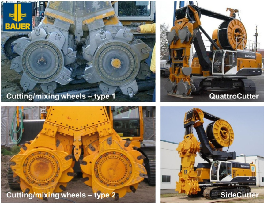
Figure 11.7 The cutting/mixing tools of the Bauer CSM system (left) and the QuattroCutter and SideCutter systems (right). (Source: From Gerresen (2012), with courtesy of Bauer).
