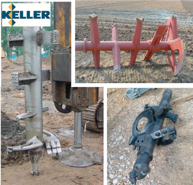
Figure 11.3 Keller wet mixing system in single shaft configuration (available tool diameter for single shaft ranging between 40 and 240 cm). (Source: From Topolnicki (2012), with courtesy of Keller).
